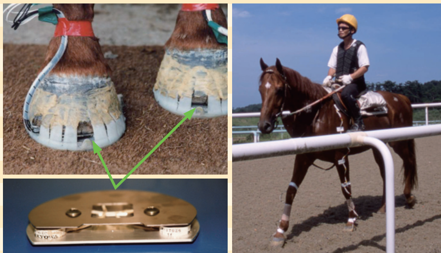
Photos: Instrumented shoe (upper left), small force plate (lower left), horse fitting instrumented shoes (right)
